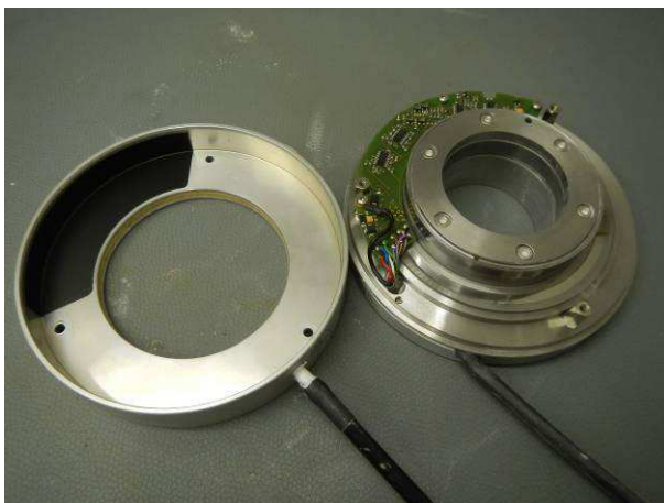
Picture 5 Incremental encoder HOGS151 DN 5000 without visible traces of dust inside after the dust test IP6X
