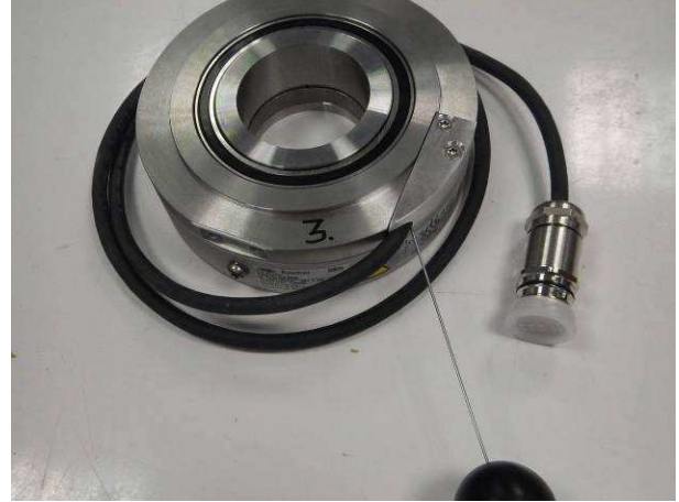
Picture 2 Incremental encoder HOGS151 DN 5000 with standardized test wire (Ø 1 mm, 1 N) during the access to hazardous parts test IP6X
