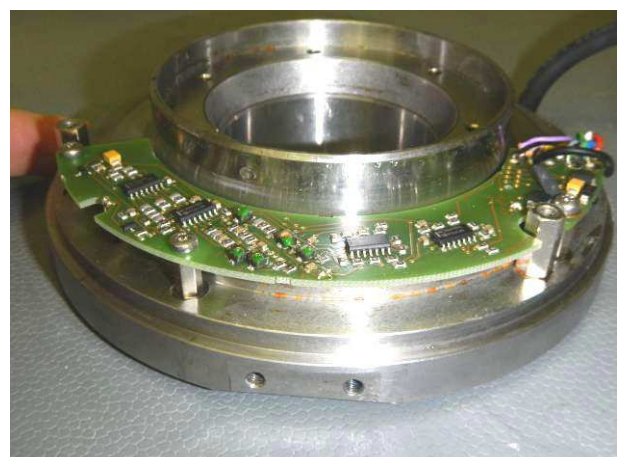
Picture 12 Incremental encoder HOGS151 DN 5000 without visible traces of water on the circuit board after the protection against splash water test IPX4
